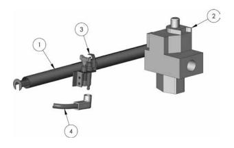
Gas Valve and Pilot, Intermittent Ignition, Current
