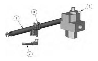
Gas Valve and Pilot, Intermittent Ignition, Current
