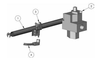
Gas Valve and Pilot, Intermittent Ignition, Current
