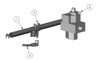
Gas Valve and Pilot, Intermittent Ignition, Current
