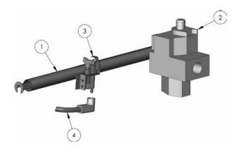
Gas Valve and Pilot, Intermittent Ignition, Current
